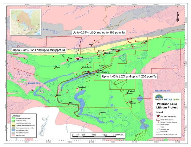
Figure 2 Paterson Lake Lithium Project geology and pegmatite occurrences map.
