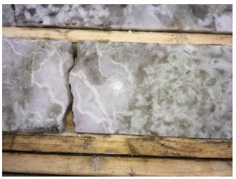
Figure 3 Pale pink to grey pollucite with white veining next to pale green spodumene at 49.5 m, PWM-18-116, West Joe Dyke.
