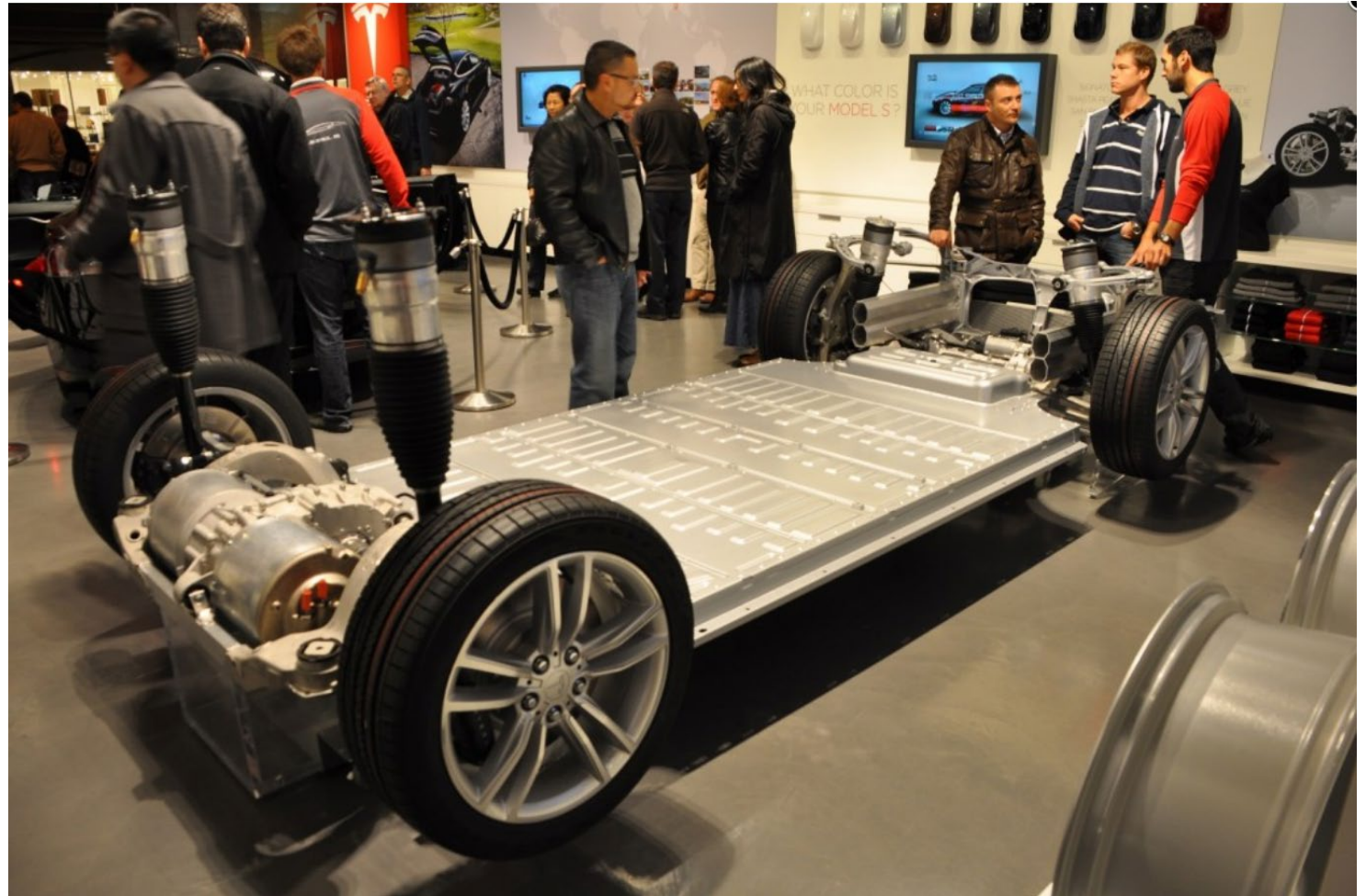
Telsa Model S lithium-ion battery pack, ( www.greencarreports.com )
