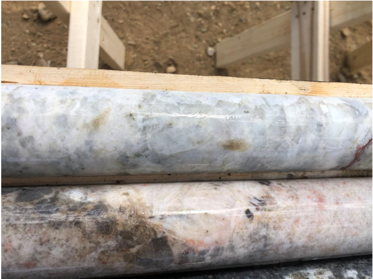
Figure 2 White spodumene at 55 m in the top row and white coarse-grained cleavelandite in the second row, PWM-22-130, West Joe Dyke
