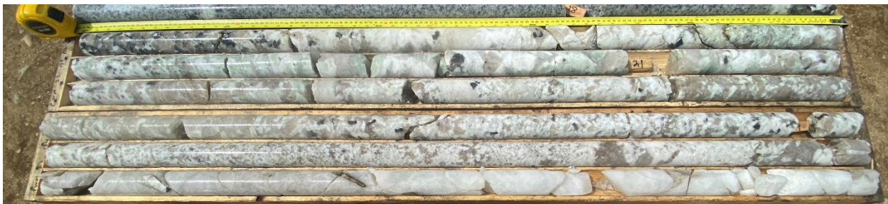
Figure 3 Abundant green spodumene in top core box and white and green spodumene in bottom box, last row is quartz core with coarse-grained spodumene, boxes 5 and 6, 20-29 m, PWM-22-134, Main Dyke.
