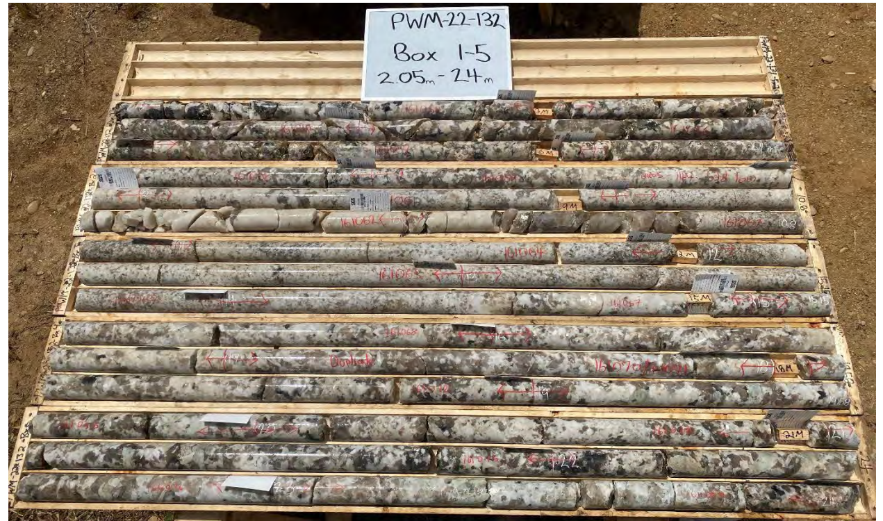
Spodumene pegmatite, Main Dyke, drill hole PWM-22-132
