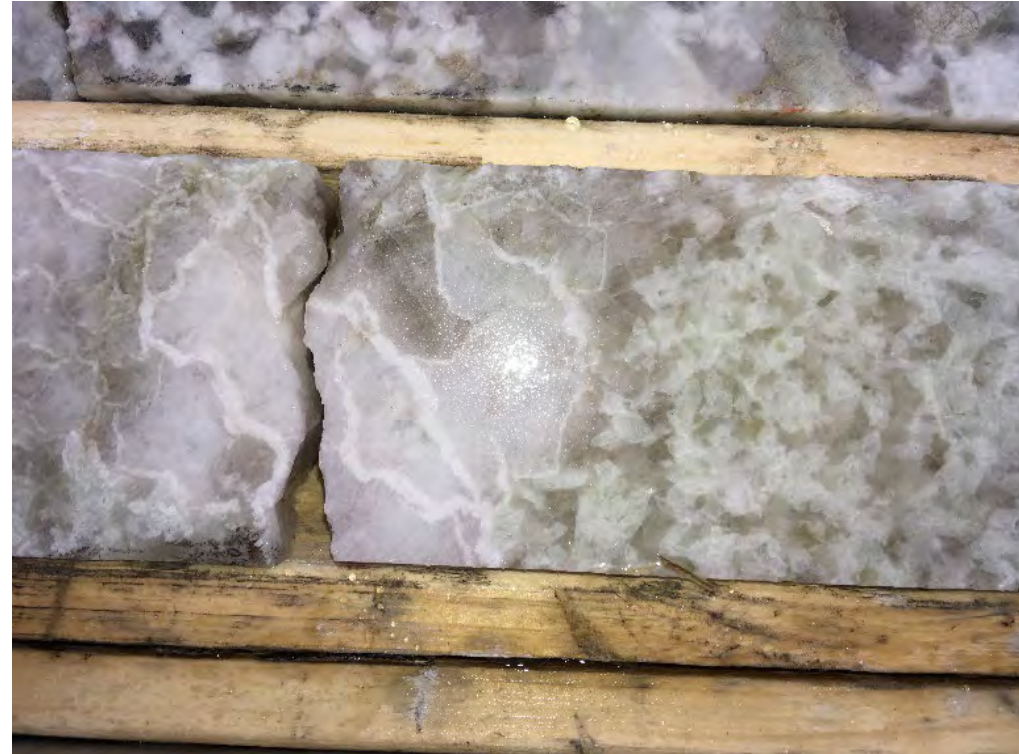
Pale pink to grey pollucite with white veining next to pale green spodumene at 49.5 m, with 2.61 % \text{Cs}_2\text{O} over 1.46 m, PWM-18-116, West Joe Dyke
