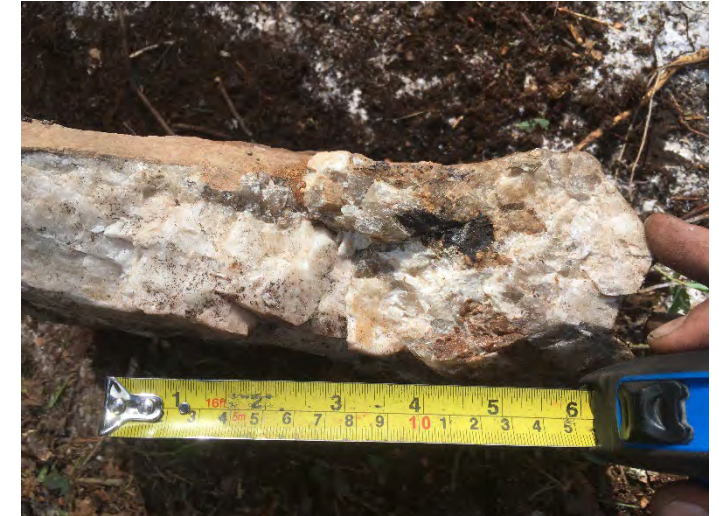
3 cm long Ta-oxide crystal, West Joe Dyke
