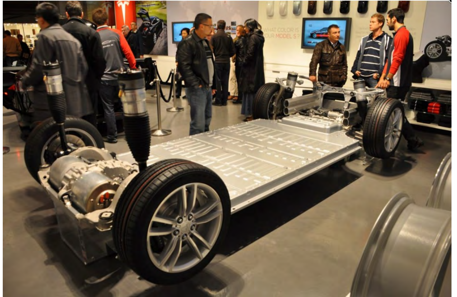
Telsa Model S lithium-ion battery pack, ( www.greencarreports.com )
