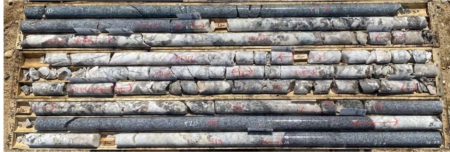
Pollucite-spodumene-Ta-oxides, pegmatite intervals 11.96 – 19.05 m, and 20.65 – 21.69 m, PWM-22-143, West Joe Dyke
