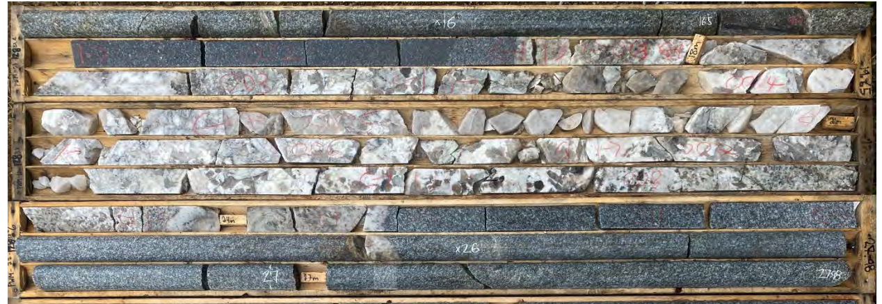
Pollucite-spodumene-Ta-oxides, pegmatite interval 17.8 – 24.4 m, 6.6 m, PWM-22-128, West Joe Dyke.
