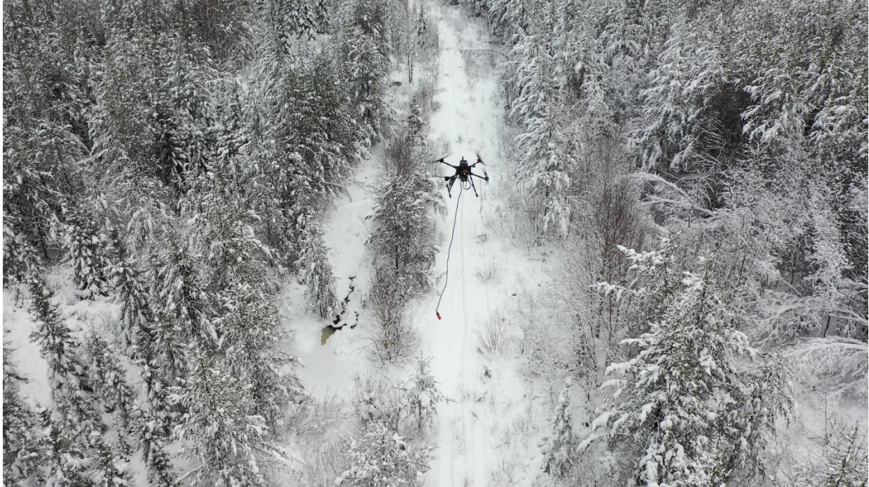
Figure 3 – Aerial image of Magnetic Drone Survey from the Case Lake Project, Ontario, Canada
