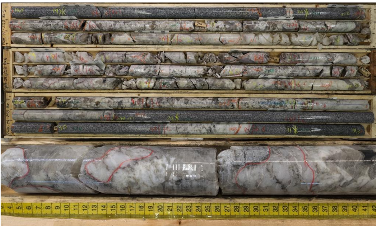
Figure 3 – Photo of drill core from PWM-24-248 displaying 8.5 meters of pollucite, spodumene, and tantalite mineralization from West Joe at the Company's Case Lake Property, Ontario, Canada
