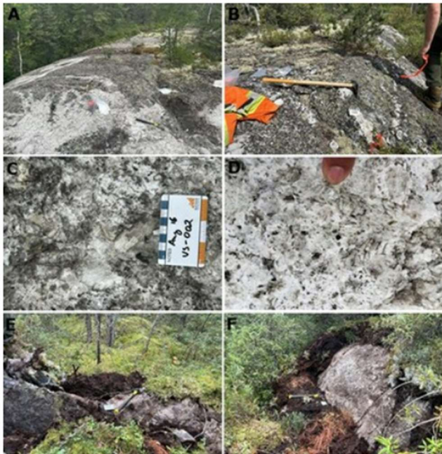
Figure 4 – Outcrop photos taken during the 2023 field exploration program at Case Lake. Figure 4A to 4C show photos taken from spodumene bearing new pegmatite in Dome Nine. Figure 4D show spodumene in the western part of the East Dike. Figures 4E was taken from new pegmatitic tonalite hosted in mafic metavolcanics in the southern part of the property. Figure 4F was taken from a new pegmatite that occurs about 500 meters north of the Northeast Dike.
