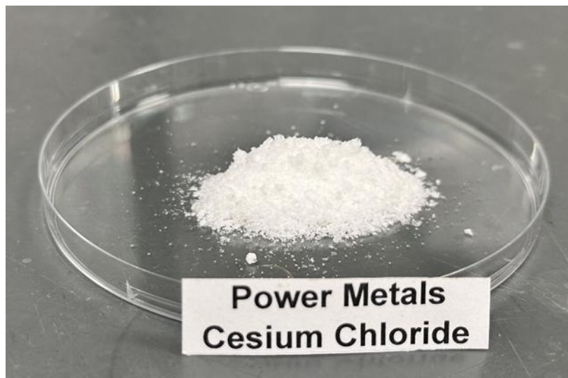
Figure 2 – Sample of 99.6% cesium chloride crystals produced from West Joe pollucite concentrate
