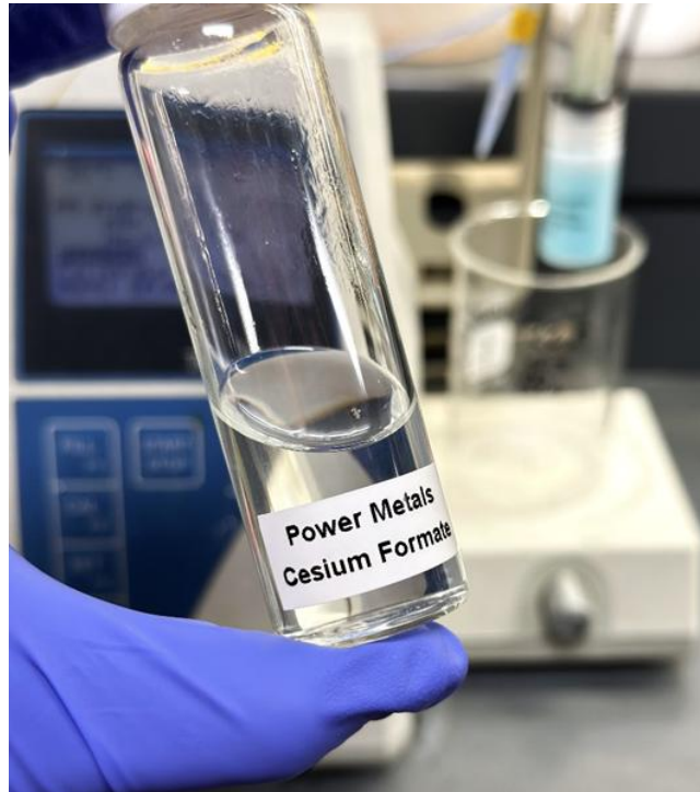
Figure 1 – Sample of 99.8% cesium formate solution with density 2.23 g/mL produced from West Joe pollucite concentrate
